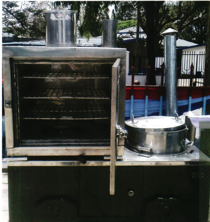
Miniaturized domestic DEFKITCH (on the right side) which is under development and the Industrial DEFKITCH loaded with oven (on the left side) which is also under development.
